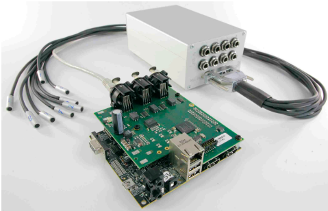
Fig. 1. Acoustic processing unit with satellite unit and 8 microphones.
